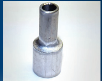
Figure 1: Non-Corrosive Flux post braze (top) vs AL CC cleaned post braze (bottom)
