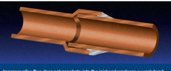
Improper alloy flow does not penetrate into the joint and produces a weak bond.
