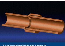
A well brazed joint begins with a proper fit between components, .001"– .003" of clearance.
