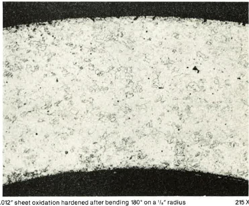
Figure 6. Recrystallized microstructure of Consil 995 after oxidation hardening (starting temper-hard-as-rolled)
